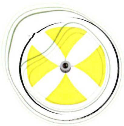
Figure 11-7 Non-uniform Electromagnetic Field Caused by Area of Weakness in Pipe Wall
