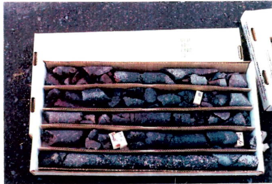
Figure 4-7 Petroleum Stained Core - B16C, 49' to 60'
