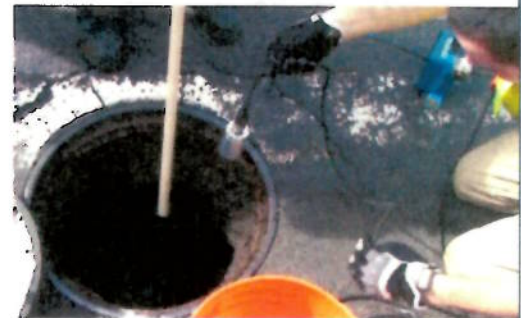
Echologics staff inserting a sensor onto a 42-inch water main.
